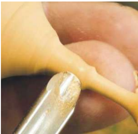
▲ Pic.22 If you want to turn thin you will have to learn to support the work with your fingers as here. The micro bevelled tool is ideal for this as it puts very little pressure on the timber
